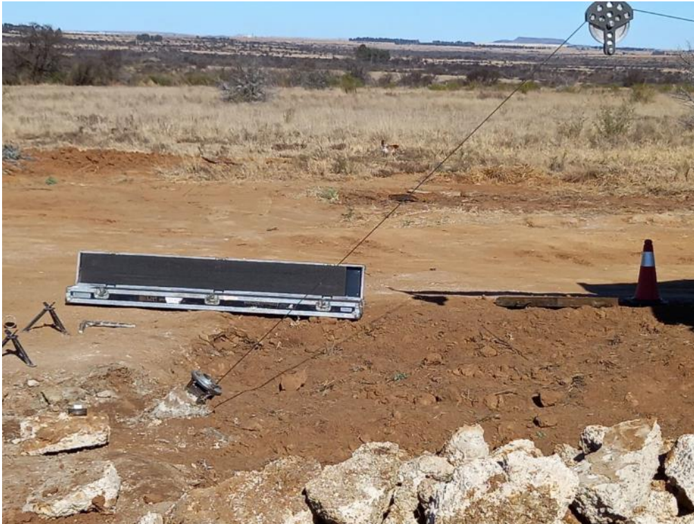
Figure 16: Well logging taking place at well P0012.
